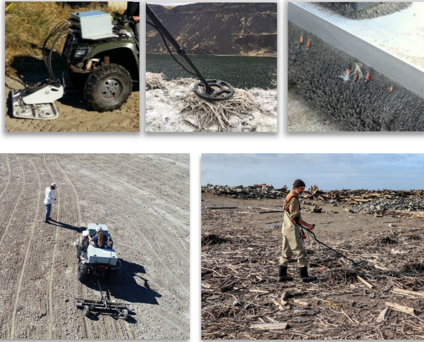
Figure A.2. Examples of equipment used to recover PIT tags from bird colonies, which include a flat-plate antenna (upper left panel), a hand-held antenna (upper middle panel), and a magnet (upper right panel). A flat-plate antenna and tow-behind magnet attached to an ATV were used to scan the Caspian tern colony on East Sand Island (lower left panel) and a hand-held antenna system was used to scan all other colonies, including the double-crested cormorant colony on East Sand Island (lower right panel).
